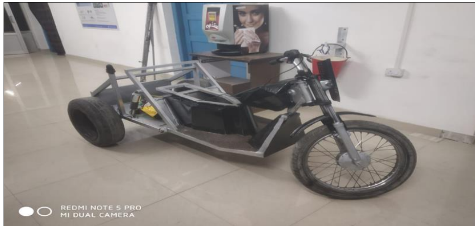
Fig 4: Delta Configuration Wheel Arrangement
