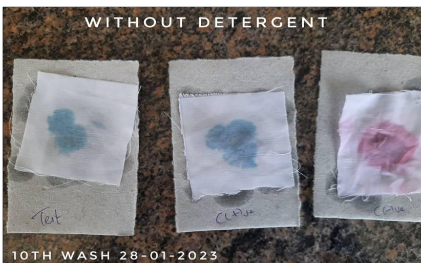
Figure 9: Benzidine test on day 10 th washed non-absorbent fabrics with plain water having normal temperature showing positive result
