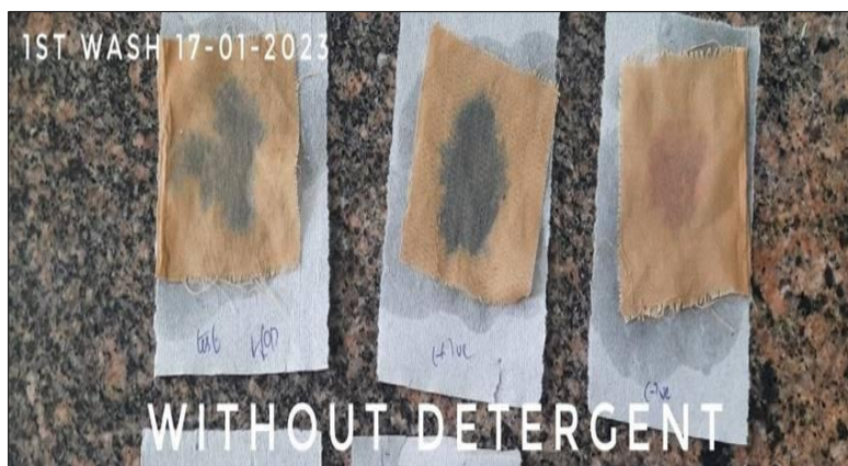
Figure 2: Benzidine test on day 1 st washed absorbent fabrics with plain water having normal temperature showing positive result
