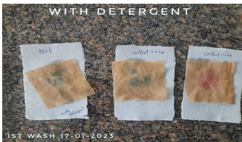
Figure 4: Benzidine test on day 1 st washed absorbent fabrics using detergent at normal temperature showing positive result
