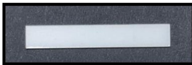
Figure 1: Plastic pattern cut using CNC
