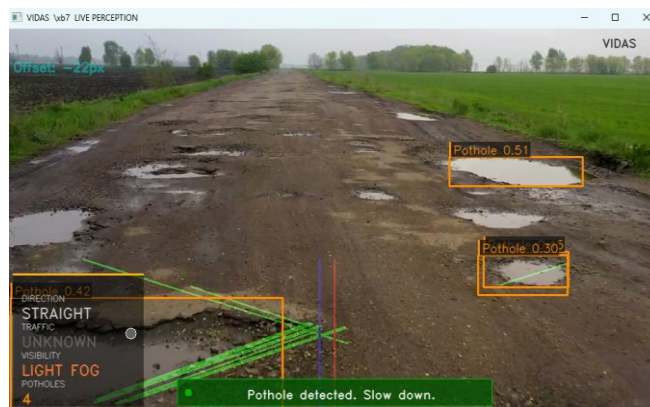
Fig. 8: Real-time integrated GUI output showing lane guidance, pothole detection, traffic signal status, fog condition, and speed display.
