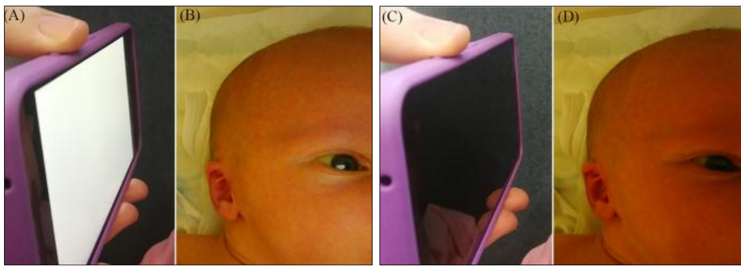
Fig 2: neoSCB app screen illumination sequence and typical flash/ no-flash sclera image pair. (A) Screen illumination on for flash image capture. (B) Example of flash image captured by app. (C) Screen illumination off for no-flash image capture. (D) Corresponding no-flash image captured by app. Media consent was provided by the parents
